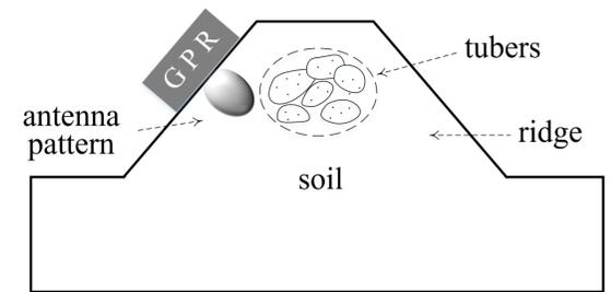
Schematic of GPR scanning on the side of a potato ridge (cross section view)
