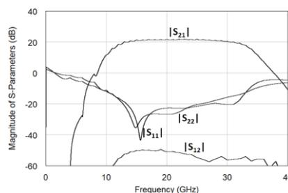
Simulation results obtained for the Hybrid Monolithic Integrated Circuit (HMIC) balanced amplifier consisting of the proposed couplers.
