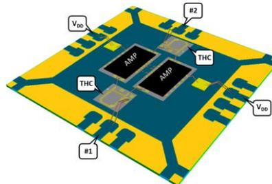
3D view of the designed balanced amplifier consisting of the proposed reduced-length tandem couplers designed on GaN substrate (THC) and amplifying stages (AMP) based on UMS CHA2069.
