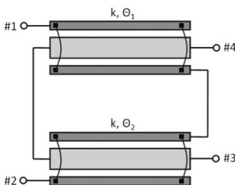
The proposed reduced-length tandem coupler composed of two three-coupled-line sections
