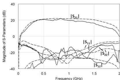
Results of simulations (dashed lines) and measurements (solid lines) of the balanced amplifier composed of the proposed tandem hybrid couplers
