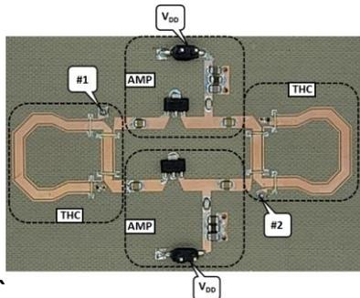
Picture of manufactured balanced amplifier consisting of proposed microstrip tandem couplers (THC) and ADL5611 amplifiers (AMP).
