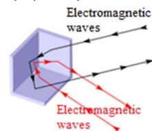
Figure 1. Concept of corner reflector
