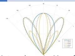
Figure 4. Antenna beams positions of DFCRA array
