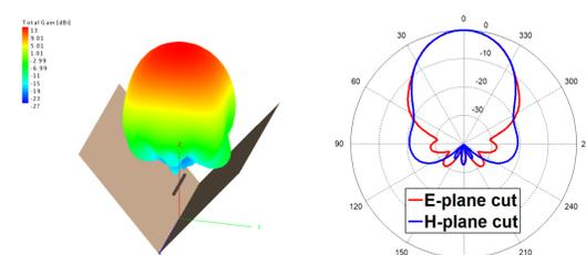
Figure 3. Total gain and radiation pattern
