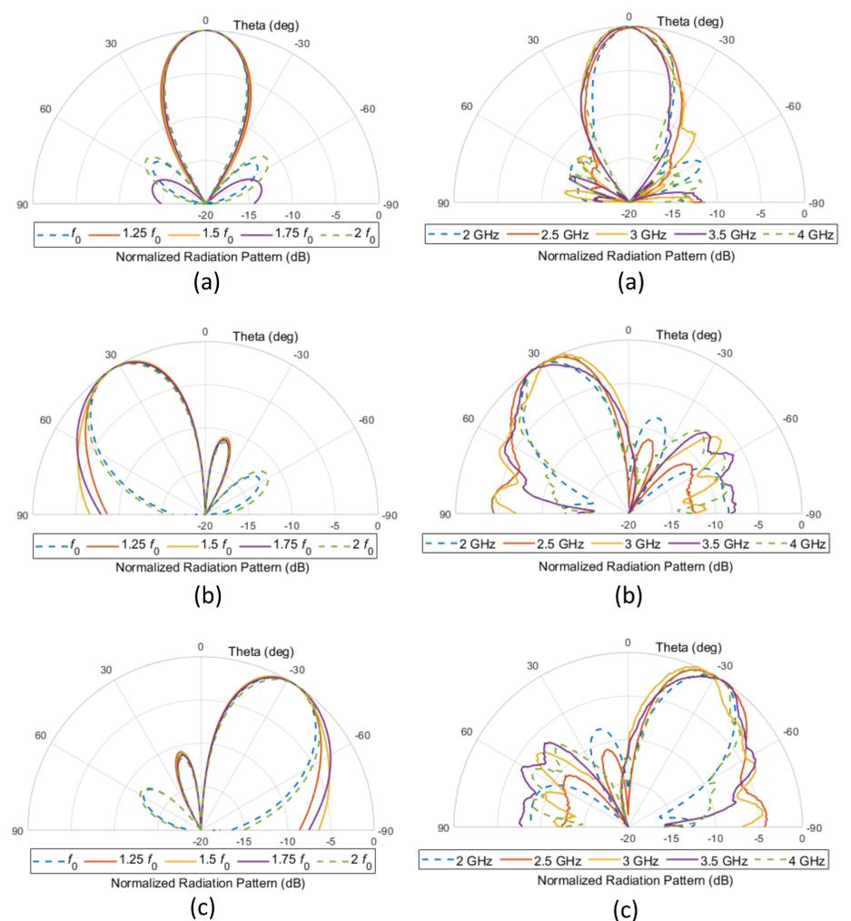
Fig. 3. Calculated broadside (a), 1L (b), and 1R (c) radiation patterns of the scalable antenna array. The radiation pattern of linearly tapered slot antenna presented in [13] was assumed for calculation purposes.
