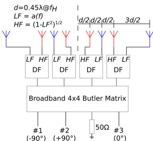
Fig. 1. Concept of three-beam scalable antenna array composed of eight radiating elements and fed through directional filters (DF) by a broadband Butler matrix.
